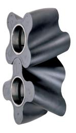
HiFlo pumps can self prime to 25' (8m), run dry, discharge to over 200psi (15 bar), pump forward or reverse and pass solids up to 2.5" (61mm).
